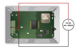
**Important**: If a wired remote controller of the AC manufacturer is connected in the same bus, communication may shut down. In case it happens, use an external power supply connected to the PS connector in our device to overcome this situation.
