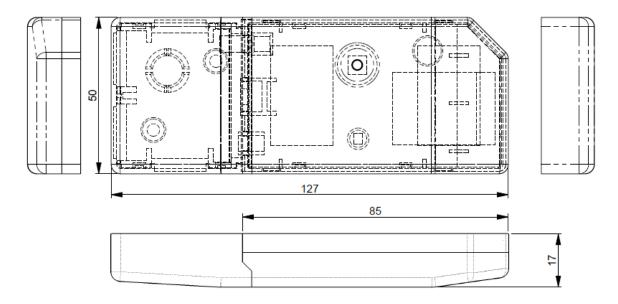
Figure 2.1 Device dimensions in mm and back view
