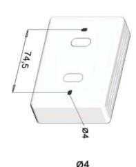
Figure 2.1 Device dimensions in mm and back view with fixing holes
