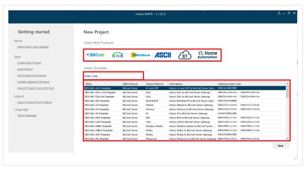
Figure 11. The three possibilities for the template selection
