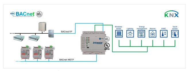
Figure 4. Integration of BACnet IP or MSTP devices into KNX control and monitoring systems
