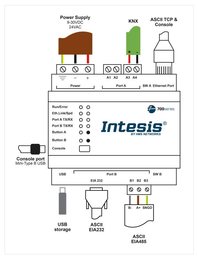
Figure 10. ASCII server to KNX
