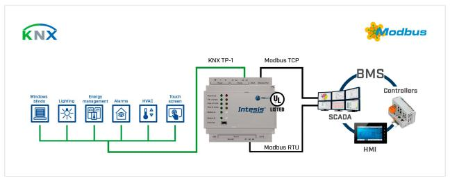
Figure 1. Integration of KNX TP devices into Modbus RTU or Modbus TCP control and monitor systems
