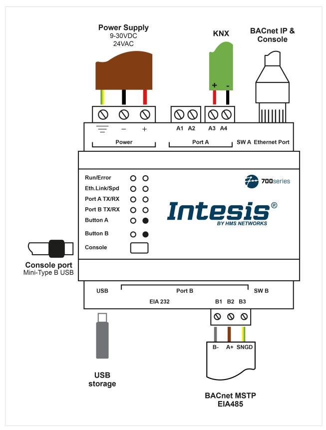
Figure 9. KNX to BACnet client
