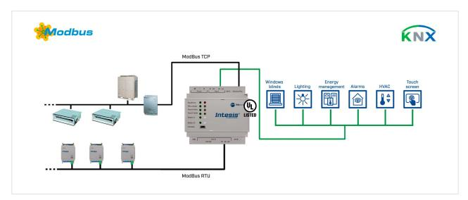
Figure 2. Integration of Modbus RTU or TCP devices into KNX control and monitoring systems
