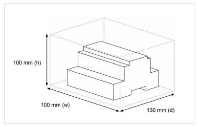
Figure 14. Space needed for connections
