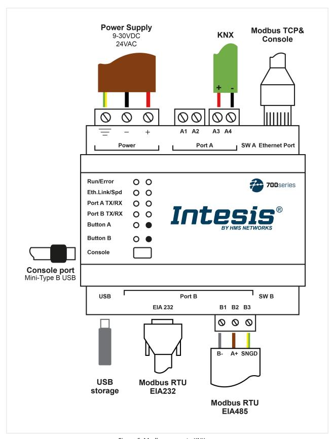
Figure 6. Modbus server to KNX  $\,$
