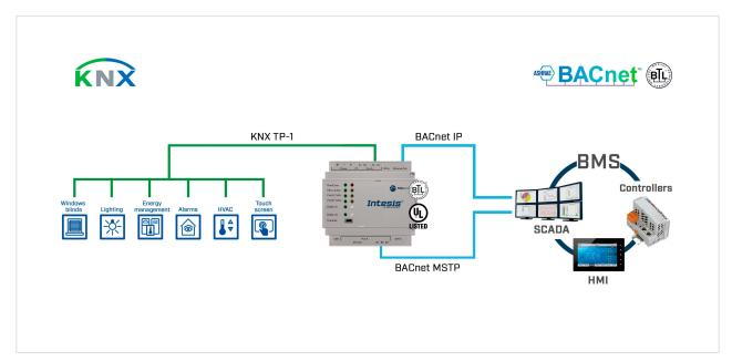
Figure 3. Integration of KNX devices into BACnet IP or BACnet MS/TP control and monitoring systems
