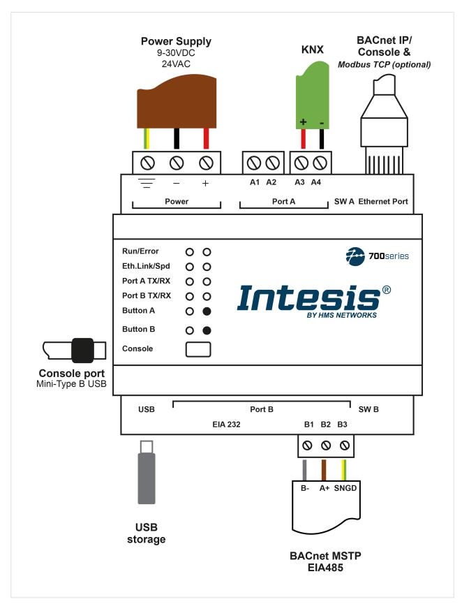
Figure 8. BACnet server to KNX
