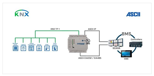
Figure 5. Integration of KNX devices into ASCII IP or ASCII serial control and monitoring systems
