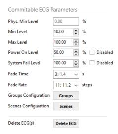
Figure 10.18 Committable ECG parameters
