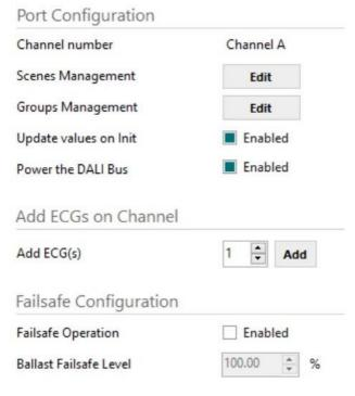
Figure 10.14 Channel parameters
