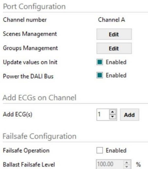
Figure 10.14 Channel parameters
