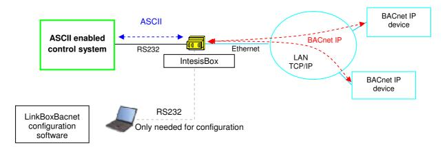
Points in BACnet can be read/written from an ASCII enabled control system using simple text messages. IntesisBox is a BACnet IP client device allowing read/write points of other BACnet IP device(s) connected to a BACnet network, and offering these point's values through its ASCII interface. ASCII interface of IntesisBox uses serial RS232 communication (baud rate configurable). For this application Daikin VRV system must be equipped with Daikin BACnet gateway DMS502B51.
