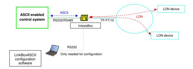
LON interface of IntesisBox reads continuously LON devices configured by polling. All the updated readings are maintained in IntesisBox's memory for immediate interaction with the ASCII system when requested. Points in LON can be read and written easily from the ASCII controller device. Each LON basic data type of network variables in LON devices can be mapped into an individual internal register, accessible through ASCII messages.
