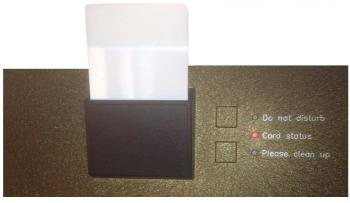
Like the card reader, the card holder is mounted horizontally. To activate the room (i.e. to switch on lights, air conditioning, power supply, etc.), the card can be inserted into the card
