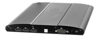
The keyboard and mouse should each be connected to a USB socket. The socket for the power supply needs to be connected to the adapter provided.
