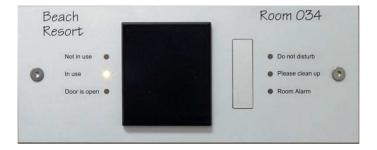
All Axesso card readers have an integrated binary output to activate DC low voltage door openers. When choosing a door opener, please make sure not to exceed the integrated switch contact's maximum current of 1A. In addition to the binary output, all card readers have two binary inputs that can be connected to any potential-free contact (e.g. door contact or card holder in a hotel environment). The function of the contact input can also be set via the parameters in the ETS application.
