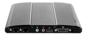
Please connect the monitor via an appropriate monitor cable (you may need to use a VGA adapter) and connect the network to the switch via a suitable patch cable. The actual card programming device should be connected to the USB connector.
