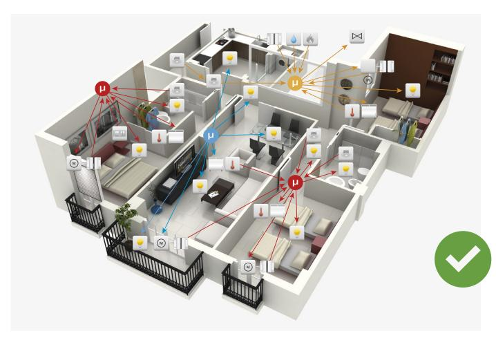
μBrick actuators are installed on either a standard DIN rail or directly on the installation base. These flexible mounting options in connection with the extremely small size offer a wide range of installation options. With μBrick actuators, the KNX installation is decentralised and no longer requires a distribution box.
