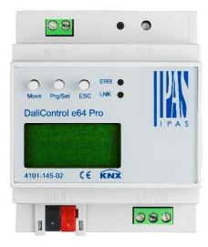
The device transforms switching and dimming commands from the connected KNX system into corresponding DALI telegrams, or status and event information from the DALI bus into KNX telegrams.
