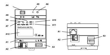
A1: RJ-45 plug for Ethernet connection
