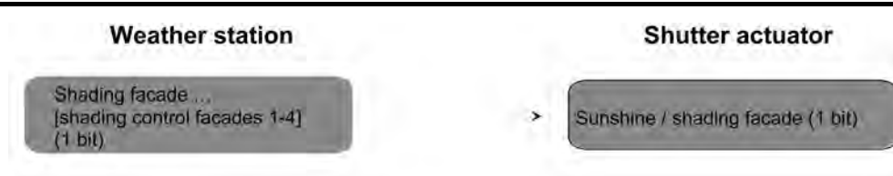
Figure 41: Programming of the communication objects for application example II.
