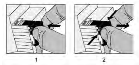
Figure 8: Installing / removing the protective cap.
