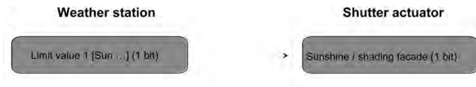
Figure 40: Programming of the communication objects for application example I.
