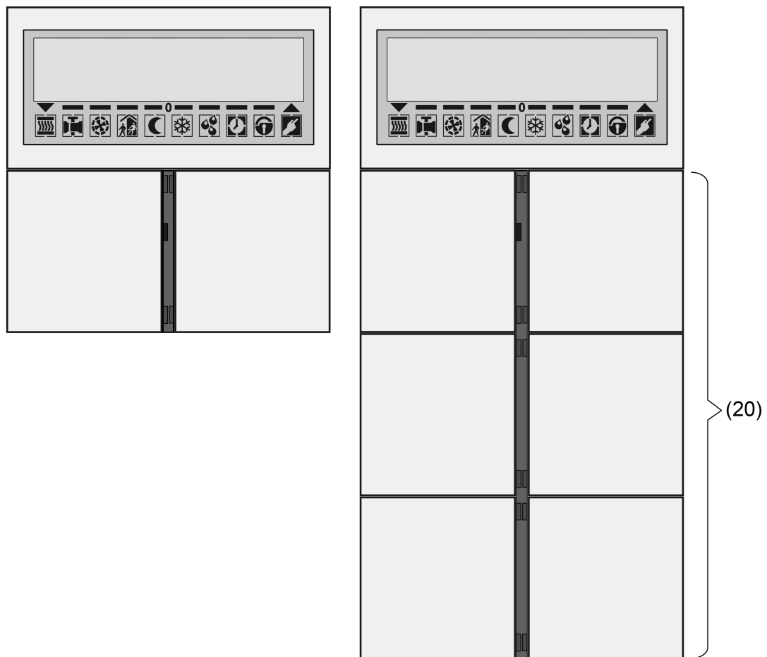
Figure 12: Arrangement of the control surfaces on the front of the device left: basic device, right: with extension module (here 4-way)
