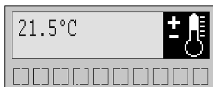
Figure 51: Example of a one-line text display with graphic symbol
