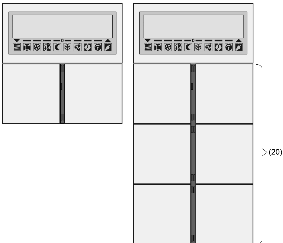
Figure 8: Arrangement of the control surfaces on the front of the device Left: basic device, right: with extension module (here 4-way)
