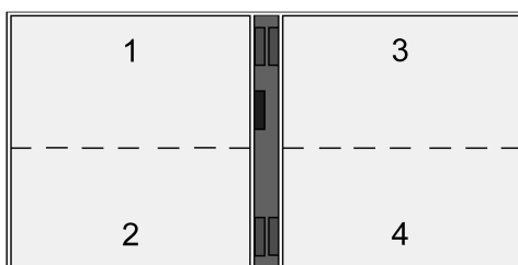
Figure 18: button arrangement "top / bottom"
