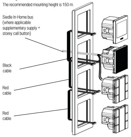
Each module is mounted in a flush-mounted appliance box according to DIN 49073. We recommend using a deep junction box for mounting. Mounting takes place using the provided supporting frames.
