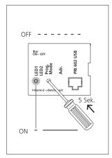
1 Activate the Plug+Play-mode at the BNG/BVNG 650-..., hold down the programming mode button for 5 seconds. LED 1 lights up permanently.
