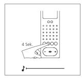
3 Hold down the light button for 4 seconds. A prolonged acknowledgement tone is audible in the receiver, the muting button flashes. A speech connection exists to the door station. The bus telephone is now in the programming mode.
