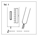
2 Lift the receiver at the first bus telephone you wish to enable for internal calls. The programming mode tone is audible.
