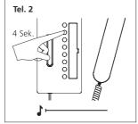
**5** Hold the light button down for 4 seconds. The acknowledgement tone is audible. Do not replace the receiver.
