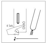
**1.1** Hold down the light button for 4 seconds. A protracted acknowledgement tone is audible in the receiver as confirmation. The bus telephone is now in the programming mode, the muting button is flashing. Do not replace the receiver until after programming has been completed at the bus telephone.
