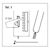
At the first bus telephone, hold down the internal call button you wish to use to call the second bus telephone for 4 seconds.
