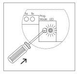
**2** Switch the BSE 650-... to the programming mode. To do this, briefly press the programming mode button with a small screwdriver. The LED flashes slowly.
