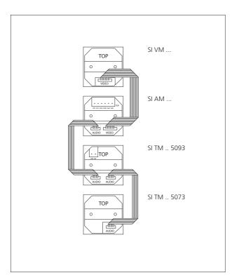
Every module is mounted in a flush-mounting junction box in compliance with DIN 49073. We recommend using a deep junction box for mounting. Mounting takes place using the provided support rings. Mounting can take place in combination or individually – horizontally or vertically.
