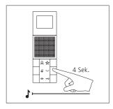
**3** Hold down the light button for 4 seconds. A protracted acknowledgement tone sounds as confirmation and the muting button begins to flash. The video indoor station establishes the speech connection to the door station. The video indoor station is now in the programming mode.
