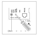
Using a small screwdriver, set the bus line rectifier to the programming mode through the opening in the cover.
