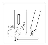
4 Hold down the light button for 4 seconds. A protracted acknowledgement tone sounds in the receiver, the muting button flashes. A speech connection exists to the door station. The bus telephone is now in the programming mode. Leave the receiver off the hook.
