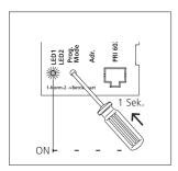
1 Switch on the programming mode. At the BNG/BVNG 650-..., press the programming mode button briefly. The LED 1 flashes in a 2-second rhythm to indicate that the programming mode is active.
