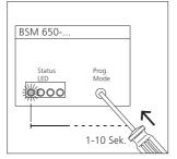
**5** The switching time for the contact is determined by the time for which the screwdriver is held down.
