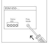
**2** Switch the BSM 650-... to the programming mode. To do this, briefly press the programming mode button using a small screwdriver.
