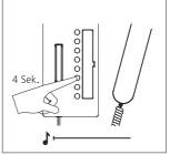
**5** At the bus telephone, hold down the button you wish to use to call the external camera for 4 seconds. Replace the receiver at the bus telephone. The button is now assigned to the external camera. The external camera can be selected at any time.
