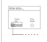
**3** Select the relevant relay by actuating the programming mode button at the BSM 650-... with the screwdriver until the required LED lights up (LED 1=relay 1).
