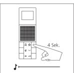
**5 Video indoor station 1:** Hold down the internal call button you wish to use to call the second device for 4 seconds.
