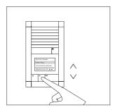
**4** At the door station, select the required name using the two arrow buttons.
