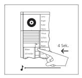
**4** Press the button to which you wish the relay to be assigned and hold down for 4 seconds.
