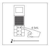
**6 Video indoor station 2:**Hold down the internal call button you wish to use to call the first device for 4 seconds.
