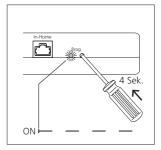
3 Press the Prog. button on the base station for 4 seconds. The LED Prog. then flashes in a one-second rhythm. The Siedle Scope/Smart Gateway Mini is now in the programming mode.
