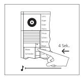
4 At the door station, hold down the required call button for 4 seconds until a protracted tone sounds at the door loudspeaker. The call button is now assigned to the bus indoor devices, no speech connection now exists.
