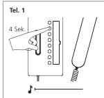
**3** Hold the light button down for 4 seconds. The acknowledgement tone is audible. Do not replace the receiver.
