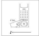
**3** Hold down the light button for 4 seconds. A prolonged acknowledgement tone is audible in the receiver, the muting button flashes. A speech connection exists to the door station. The bus telephone is now in the programming mode.
