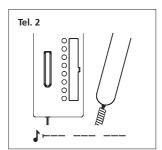
**4** Lift the receiver at the second bus telephone you wish to enable for internal calls. The programming mode tone is audible.
