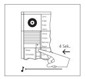
4 At the door station, hold down the required call button for 4 seconds until a protracted tone sounds at the door loudspeaker. The call button is now assigned to the bus indoor devices, no speech connection now exists.
