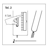
**4** Lift the receiver at the second bus telephone which you wish to program. Hold down the light button for 4 seconds. Do not replace the receiver!
