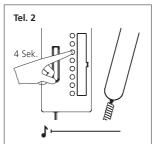
At the second bus telephone, hold down the internal call button you wish to use to call the first bus telephone for 4 seconds. A protracted tone is audible.
