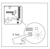
2 At the BVA 650-... hold the programming button down for 4 seconds. After this, the status LED flashes at short intervals as long as the programming mode is active.
