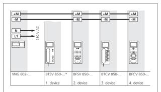
A maximum of 3 BTSV/BFSV/BTCV/BFCV 850-... units can be supplied by a NG 602-... line rectifier. The maximum current of the 30 V DC direct voltage from the VNG 602-... is 1100 mA. The specified ranges only apply to the external power supply to the devices, not to the ranges of the In-Home bus. Ranges applicable for J-Y(ST)Y or YR installation cable with 0.8 mm core diameter! Only bus indoor devices which are located in the same line can be supplied by one line rectifier.
