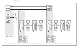
A maximum of 1 BTSV/BFSV/BTCV/BFCV 850-... unit can be supplied by a NG 602-... line rectifier. The maximum current of the 24 V DC direct voltage at the NG 602-... is 300 mA. If several bus telephones have to be simultaneously rung using one bell button, each BTSV/BFSV/BTCV/BFCV 850-... must have its own NG 602-... Alternatively, up to 3 bus telephones with colour monitor can be supplied from a video line rectifier VNG 602-...
