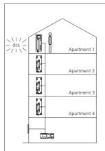
2 Set up the bus telephone in apartment 1 with the receiver in place, the storey call sounds as an acknowledgement tone and the LED of the muting button flashes. Bus telephone 1 is assigned to button 1.
