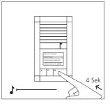
5 When the selected name is shown in the display, hold down the OK button on the DRM 612-... for 4 seconds until a protracted tone is audible at the door loudspeaker. The selected name is now assigned to the bus telephone. The speech connection is interrupted. If the name was already programmed, the OK button must be pressed 2x.
