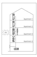
**4** Set up the bus telephone in apartment 3 with the receiver in place, the storey call sounds as an acknowledgement tone and the LED of the muting button flashes.
