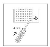
4 Hold down the programming button of the bus secondary signal unit through the opening in the louvre for 4 seconds. A brief acknowledgement tone is audible.
