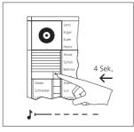
2 At the door station, hold down the light/programming button for 4 seconds. A protracted acknowledgement tone is then audible which is repeated every 5 seconds as long as the programming mode remains active.
