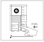
**5** At the door station, hold down the required call button for 4 seconds until a protracted tone sounds at the door loudspeaker.
