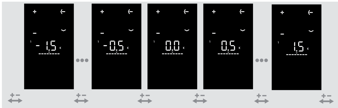
Figure 26: Setting the setpoint shift
