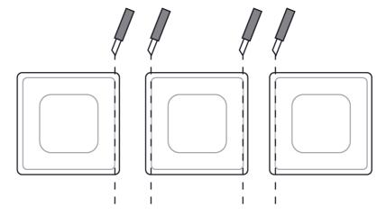
Figure 3: Cutting the adhesive pads for multiple combinations
