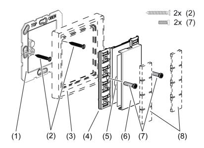
Figure 1: 4-gang radio wall transmitter module
