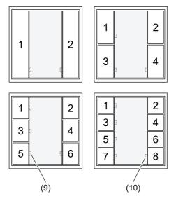
Figure 2: Button assignment of wall transmitter module 1-gang, 2-gang, 3-gang and 4-gang
