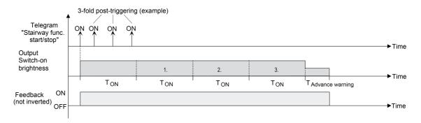
Figure 51: Time extension of the staircase function
