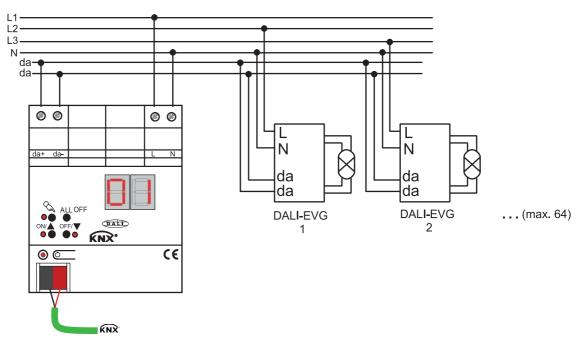
Figure 2: Electrical connection of mains voltage and the DALI interface
