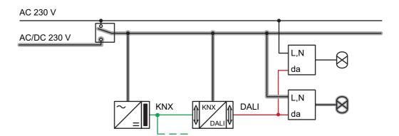
Figure 6: Electrical connection diagram in an emergency lighting system - KNX power supply, DALI emergency lights and DALI Gateway integrated into the emergency power supply (recommended installation)
