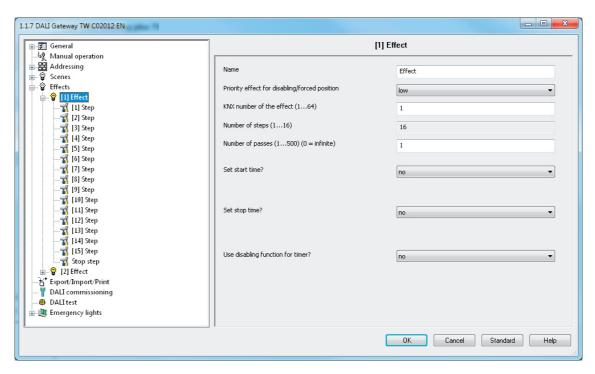
Figure 55: Configuration page of an effect as an example with 15 created effect steps and stop step
