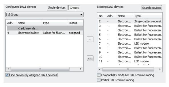
Figure 68: Operating device assigned to a group
