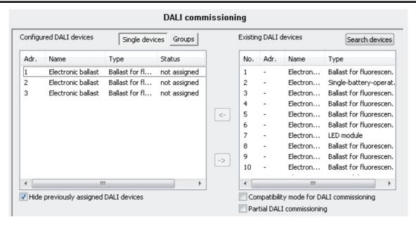
Figure 72: Operating device assigned to a programmed single device
