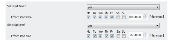
Figure 60: Example of an effect configuration with start and stop time for the timer (here: automatic starting at 8:00 and stopping 16:00 on Mon...Fri)
