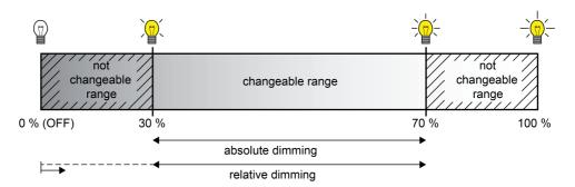
Figure 31: Example of a dimmable brightness range
