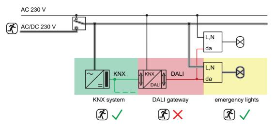
Figure 17: Example of a central supply - DALI operating devices and KNX system integrated into the emergency power supply
