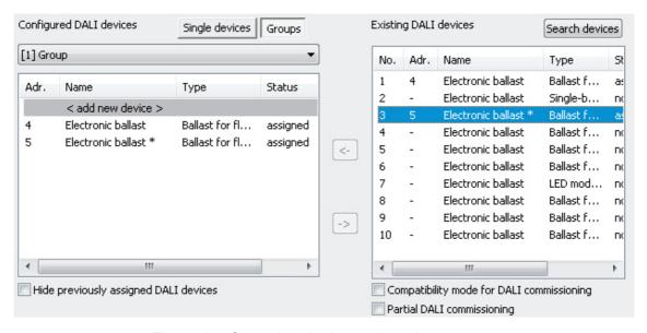
Figure 69: Operating device assigned to a group Here: Electronic ballast with the address 3 is assigned to multiple groups.
