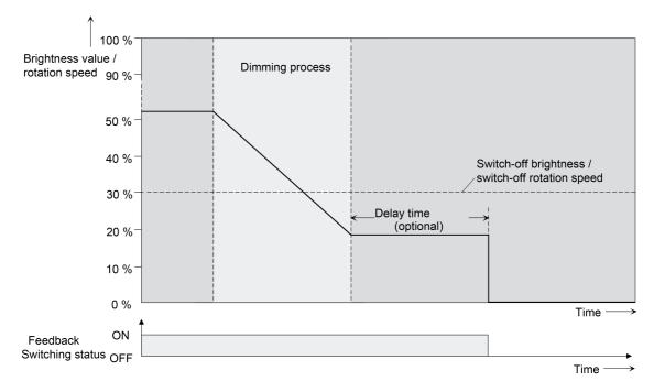
Figure 41: Dimming and switching behaviour of the automatic switch-off function
