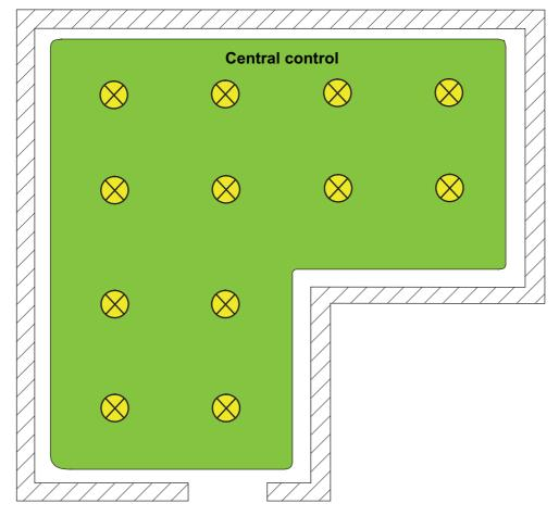
Figure 10: Example of a master control (broadcast) - Only one group
