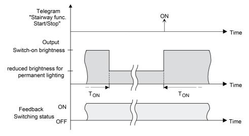
Figure 49: The continuous lighting of the staircase function without soft functions
