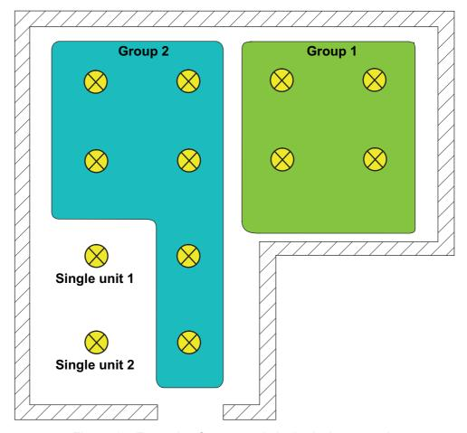
Figure 13: Example of group and single device control
