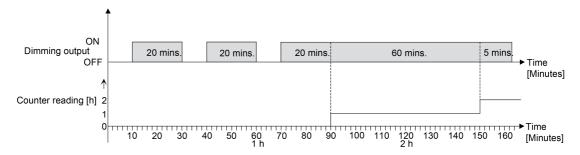
Figure 52: Function of the operating hours counter (using the example of an up-counter)
