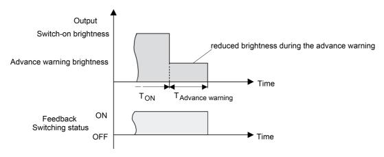
Figure 47: The pre-warning function of the staircase function without soft OFF function
