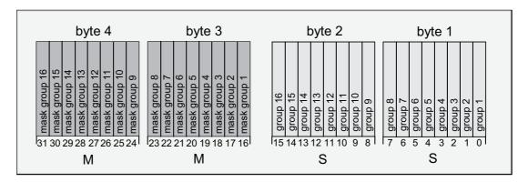
Figure 28: Structure of the objects of the collective feedback, using the example of the object for Groups 1-16
