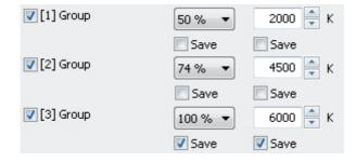
Figure 54: Example of a group assignment to a scene with brightness values and colour temperature values
