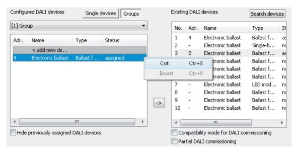
Figure 71: Moving assigned devices to another group by cutting and pasting
