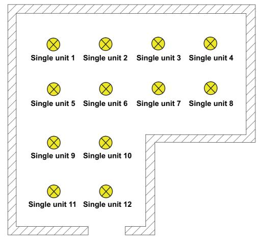
Figure 14: Example of single device control - All the DALI operating devices can be controlled individually
