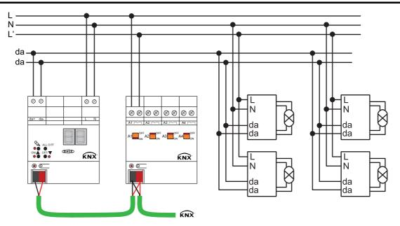
Figure 29: Example of a connection diagram for standby switch-off by a KNX switching actuator
