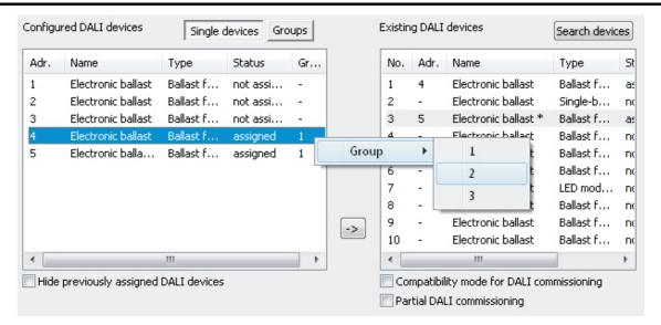
Figure 70: Directly moving assigned devices to another group
