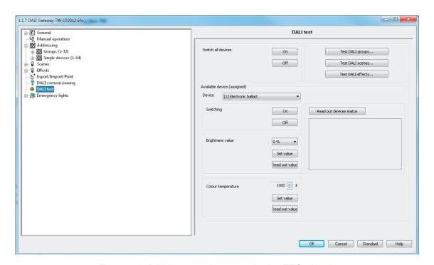
Figure 79: DALI test environment in the ETS plug-in
