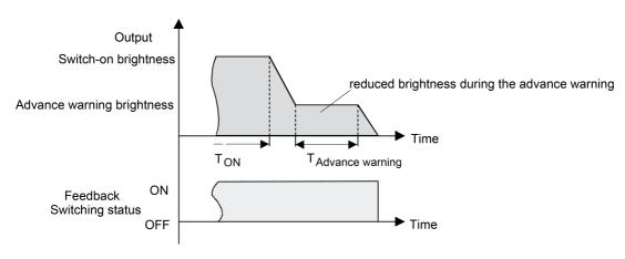
Figure 48: The pre-warning function of the staircase function with soft OFF function (as an example with minimum brightness = 0 %)
