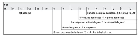
Figure 27: Telegram structure, 2-byte KNX error status
