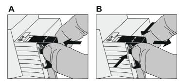
Figure 7: Installing / removing the protective cap
