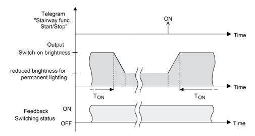
Figure 50: The continuous lighting of the staircase function with soft OFF functions
