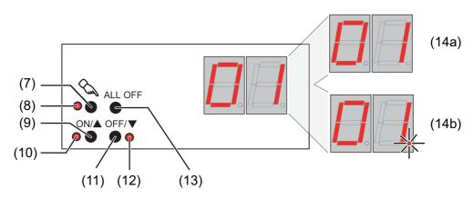
Figure 8: Controls and indicators for manual control
