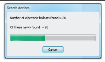
Figure 65: Example of search progress during a DALI operating device search
