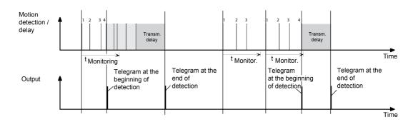
Figure 23: Motion evaluation with the detector
