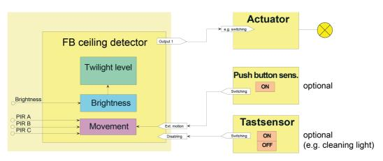
Figure 19: Application example of the application ceiling detector
