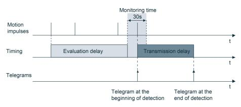
Figure 38: Evaluation delay with ongoing motion
