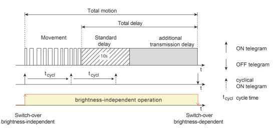
Figure 35: Total motion with motion detection, standard delay and additional transmission delay
