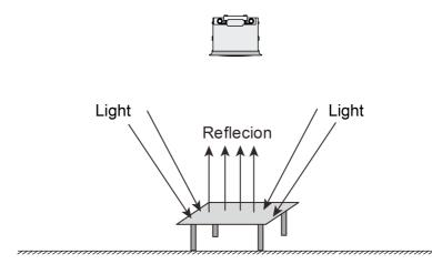
Figure 16: Brightness determination by measuring reflected mixed light composed of artificial light and daylight
