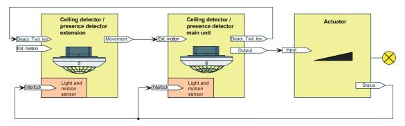
Figure 32: Application example with twilight level evaluation in the main unit and extensions Universal solution for all data formats
