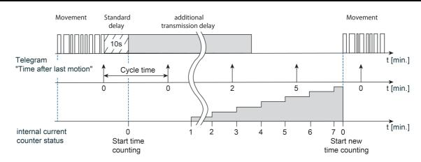
Figure 41: Measurement of the time period after last motion
