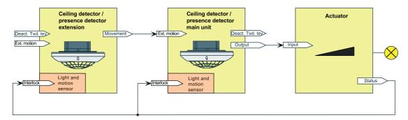
Figure 29: Application example of main unit and extension without twilight level evaluation
