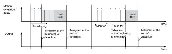
Figure 40: Motion evaluation with the detector
