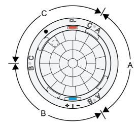
Figure 6: Labelling of the PIR sectors on the device
