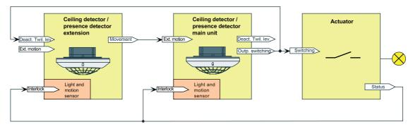
Figure 31: Application example with twilight level evaluation in the main unit and extensions for the data format "Switching"
