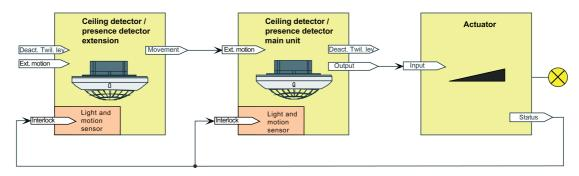
Figure 30: Application example of main unit and extension with twilight level evaluation in the main unit
