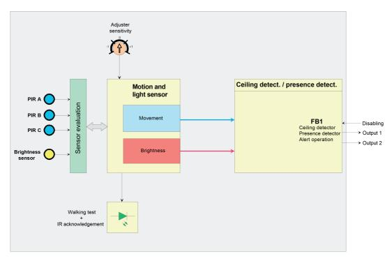
Figure 14: Block diagram of all device functions
