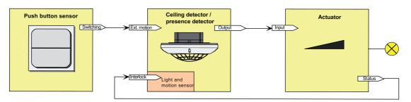
Figure 28: Application example of single device with external motion detection
