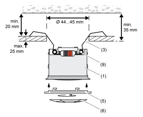
Figure 8: Mounting in a suspended ceiling
