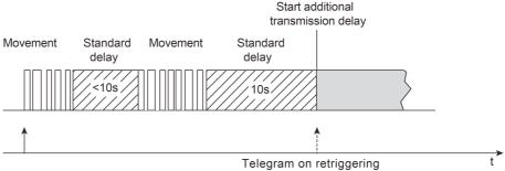
Figure 37: Triggering of a telegram when retriggering
