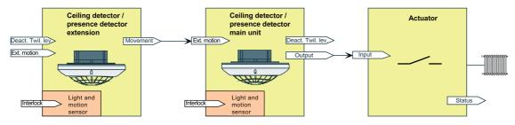
Figure 34: Application example without twilight level evaluation in the main unit and extensions
