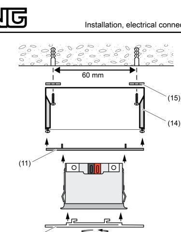
Figure 11: Mounting in the flush-mounted housing (accessories)
