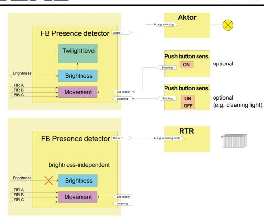
Figure 21: Application examples of the application presence detector
