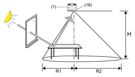
Figure 7: Alignment of the brightness sensor
