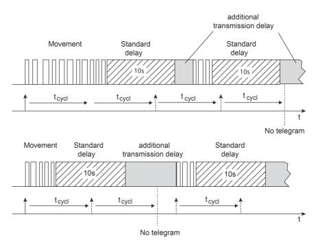
Figure 36: Cyclical transmission during a motion detection
