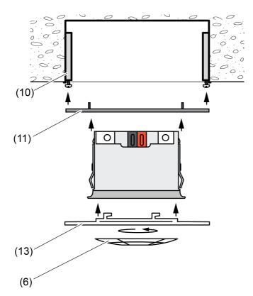
Figure 10: Mounting in a flush-mounted/cavity wall appliance box
