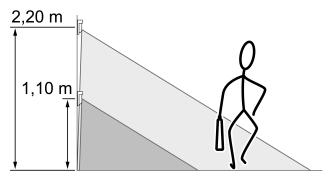
Figure 8: Detection field and mounting height
