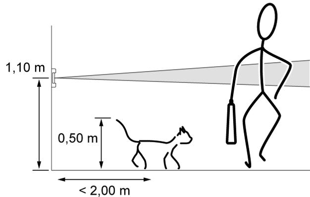
Figure 11: Detection field and mounting height
