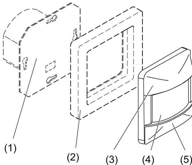
Figure 1: Device components
