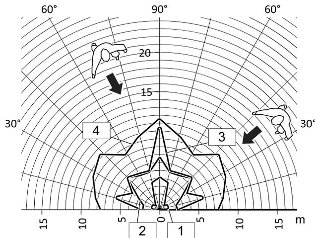
Figure 10: Range with radial direction of motion
