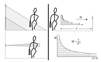
Figure 4: Detection of heat sources – detection field geometry and distance (photometric distance law)
