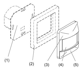
Figure 1: Device components
