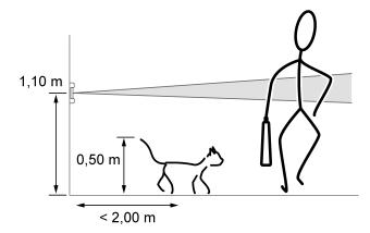
Figure 11: Detection field and mounting height
