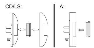
Figure 17: Mounting, cover, ranges LS/CD and A ranges
