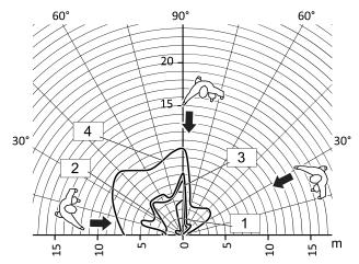
Figure 14: Range with radial direction of motion
