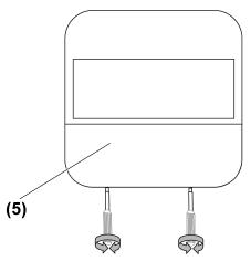
Figure 15: Dismounting of slide switch
