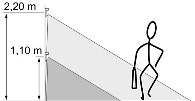
Figure 8: Detection field and mounting height
