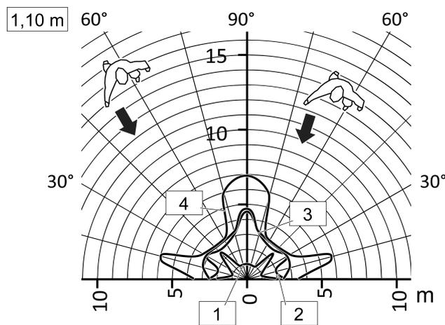
Figure 12: Range with radial direction of motion, mounting height 1.10 m
