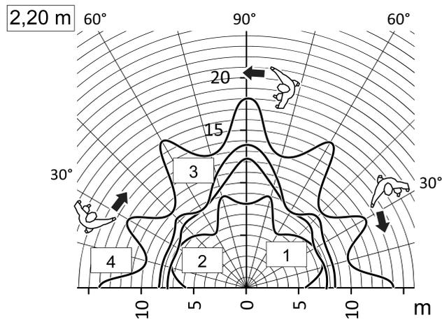
Figure 9: Range with tangential direction of motion, mounting height 2.20 m
