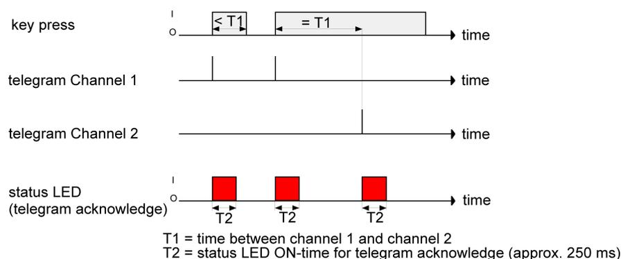
Image 16: Example for operation concept "Channel 1 and channel 2"
