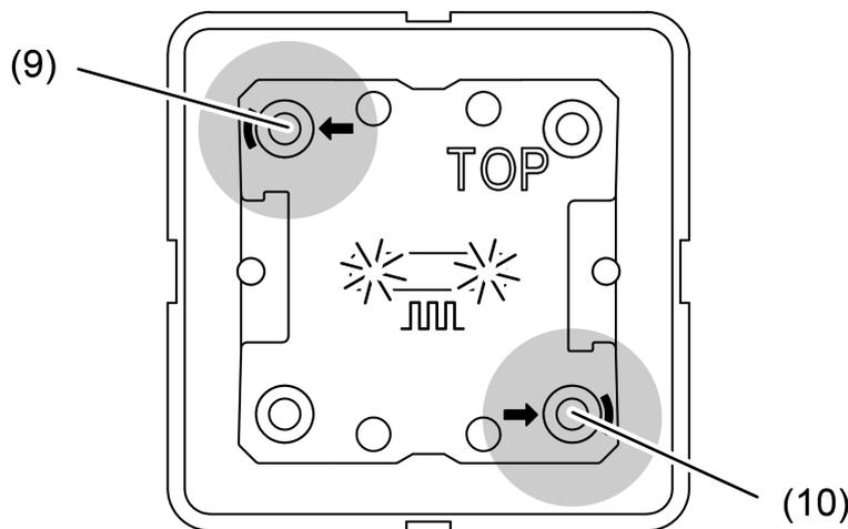
Image 8: Buttons for activating Programming mode
