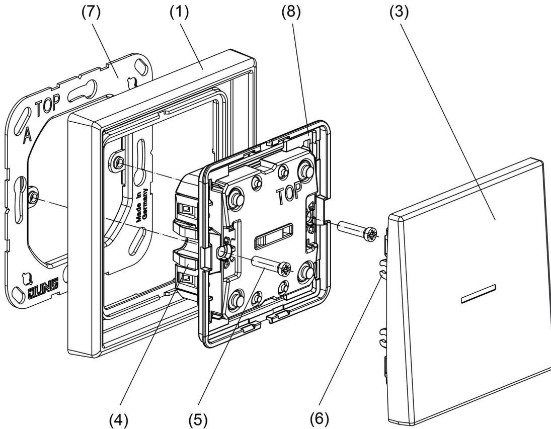
Image 3: Fitting the device
