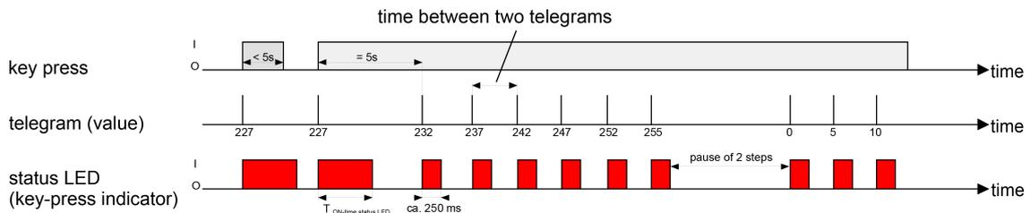
Image 14: Example of value adjustment with value range overflow
