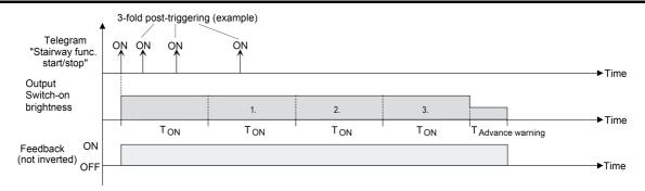
Figure 29: Time extension of the staircase function
