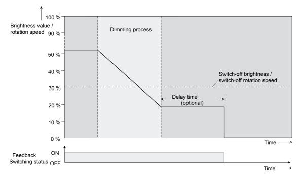
Figure 20: Dimming and switching behaviour of the automatic switch-off function
