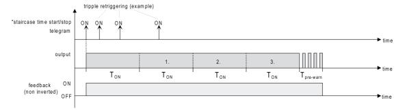
Figure 35: Time extension of the staircase function
