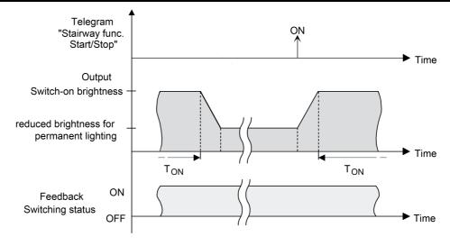
Figure 28: The continuous lighting of the staircase function with soft OFF functions
