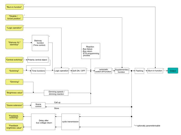
Figure 10: Function diagram of the dimming channels
