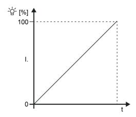
Figure 13: Linear dimming characteristic
