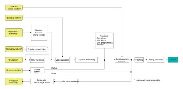
Figure 31: Function diagram of the switching channels
