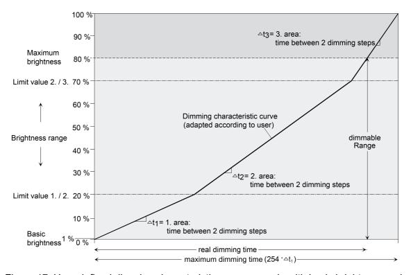
Figure 17: User-defined dimming characteristic as an example with basic brightness and maximum brightness (example with 3 areas)
