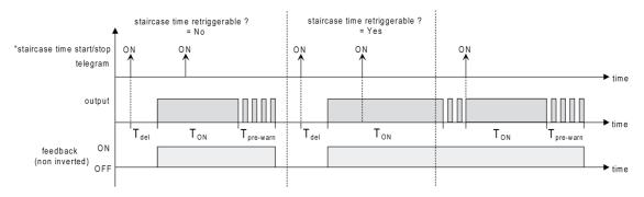
Figure 32: Switch-on behaviour of the staircase function
