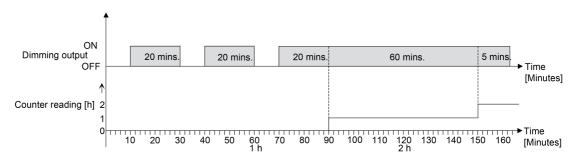
Figure 37: Function of the operating hours counter (using the example of an up-counter)
