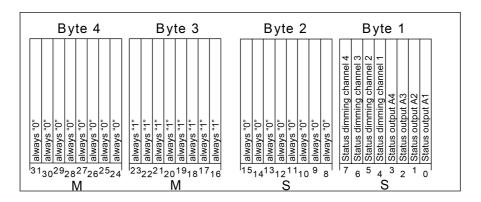
Figure 9: Object structure of the collective feedback
