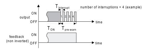
Figure 34: The pre-warning function of the staircase function (example)
