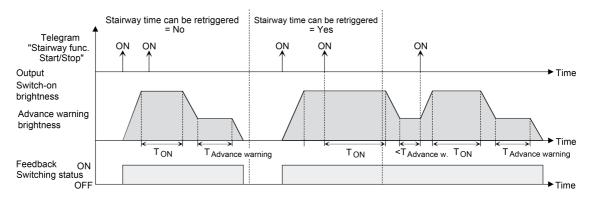
Figure 22: Switch-on behaviour of the staircase function with soft functions (for example with minimum brightness = 0 %)
