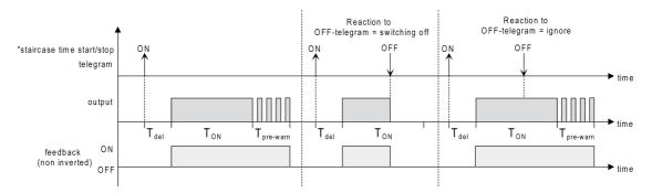
Figure 33: Switch-off behaviour of the staircase function
