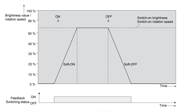
Figure 19: Dimming behaviour of the soft ON/OFF functions (as an example)
