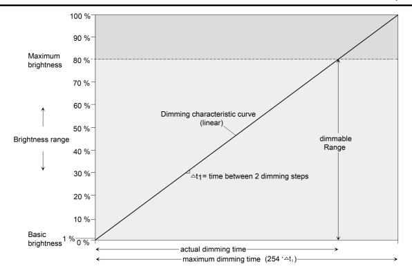
Figure 15: Linear dimming characteristic as an example with basic brightness and maximum brightness
