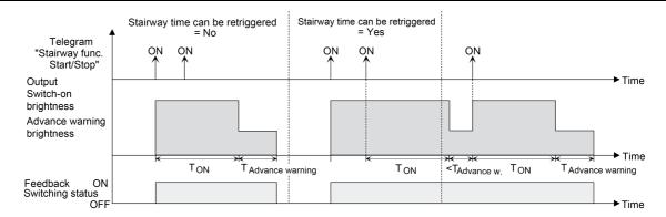
Figure 21: Switch-on behaviour of the staircase function without soft functions
