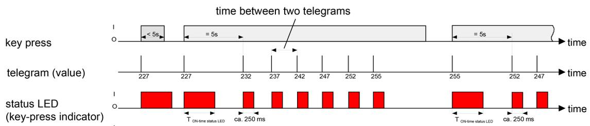
Image 8: Example of value adjustment without value range overflow
