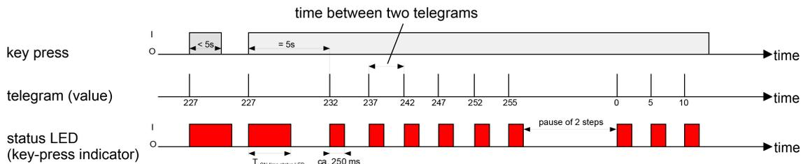
Image 9: Example of value adjustment with value range overflow
