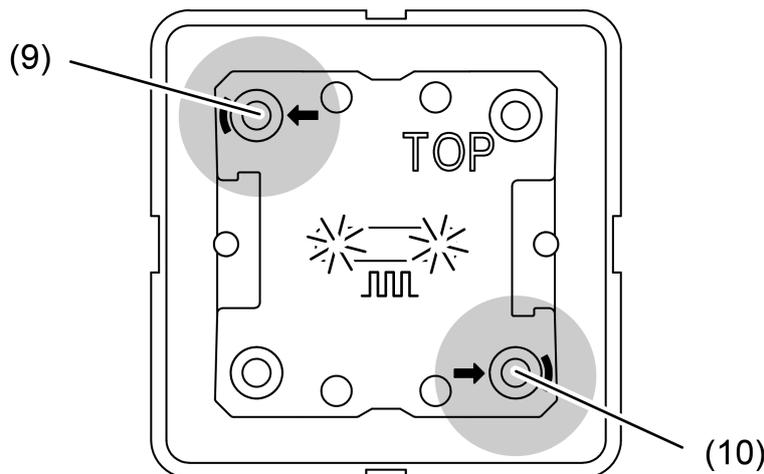
Image 6: Buttons for activating Programming mode
