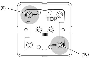
Image 8: Buttons for activating Programming mode
