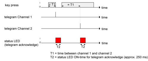
Image 15: Example of operation concept "Channel 1 or Channel 2"
