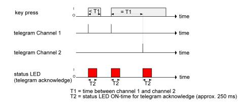
Image 16: Example for operation concept "Channel 1 and channel 2"
