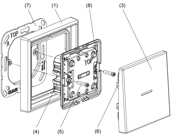
Image 3: Fitting the device
