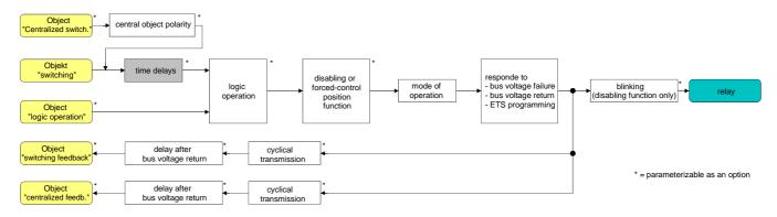
Fig.9: Functional diagram of the time delays
