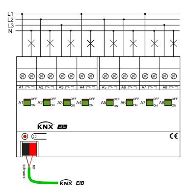
Fig. 1: Electrical connection
