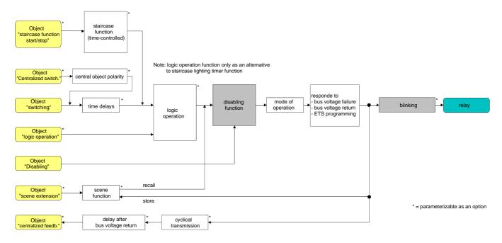
Fig. 19: Functional diagram of the disabling function
