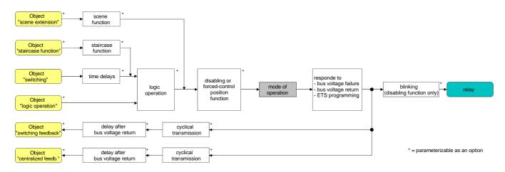
Fig. 6: Functional diagram "Mode of operation"
