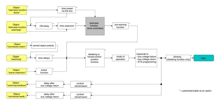
Fig. 10: Functional diagram of the staircase function
