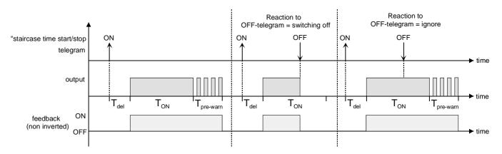
Fig. 12: Switch-off behaviour of the staircase function
