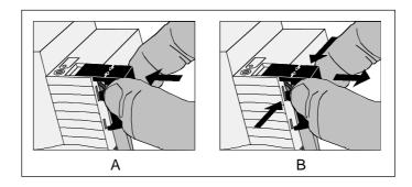
Fig. 2: Installing / removing the protective cap
