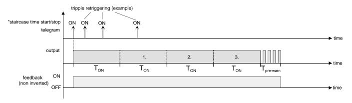
Fig. 14: Time extension for staircase lighting function
