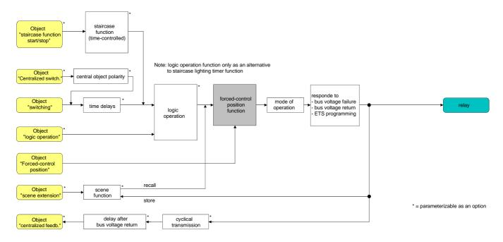
Fig. 20: Functional diagram of the forced-control position function
