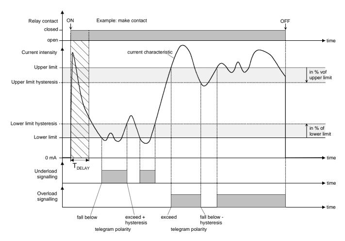
Fig. 17: Load monitoring with fixed load limits (exemplary current characteristic)
