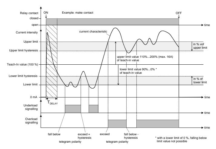
Fig. 18: Load monitoring with teach-in (exemplary current characteristic)
