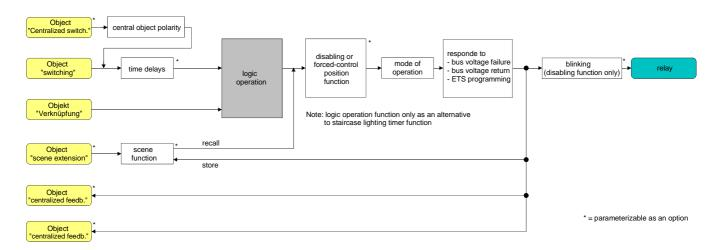
Fig. 21: Functional diagram of the logic function
