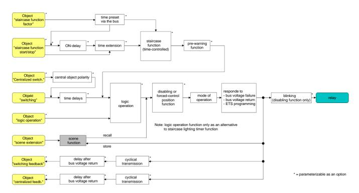
Fig. 15: Functional diagram of the scene function
