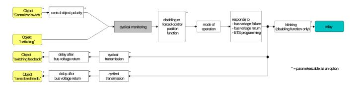
Fig. 8: Functional diagram of cyclical monitoring function
