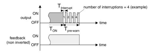
Fig.13: The pre-warning function of the staircase function
