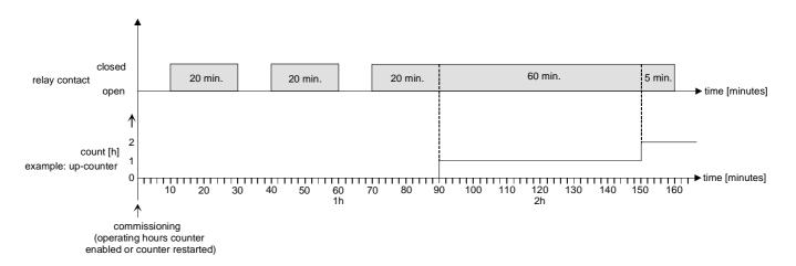
Fig. 16: Functional principle of the operating hours counter
