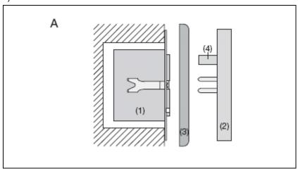
The connection terminals of the insert must be down. The extension insert can only be used in combination with the short-stroke pushbutton. Plug
