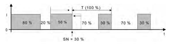
Figure 61: Command value change e.g. from 80 % to 30 % during the opening phase of the valve (opening phase too long)
