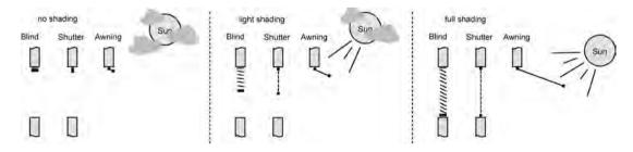
Figure 37: Sun protection principles (example)
