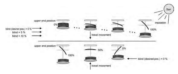
Figure 34: Example of slat positioning with the blind in upper end position (typical of slat type 1.)
