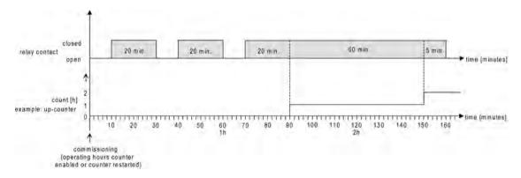
Figure 23: Functional principle of the operating hours counter
