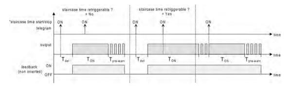
Figure 18: Switch-on behaviour of the staircase function
