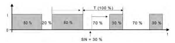
Figure 60: Command value change e.g. from 80 % to 30 % during the closing phase of the valve
