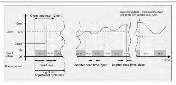
Figure 66: Idealised curve of the valve stroke: example for an initial command value of approx. 60 % for a valve closed when deenergized
