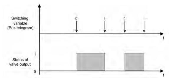
Figure 53: Conversion of a switching command value into an output signal with valve drives that are open when deenergized (example)
