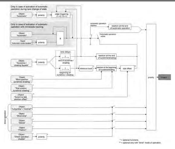
Figure 41: Function diagram illustrating the enlarged sun protection
