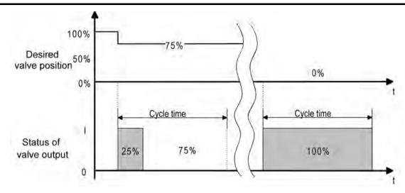
Figure 54: Conversion of a constant valve nominal position into an output signal with valve drives that are open when deenergized (example)
