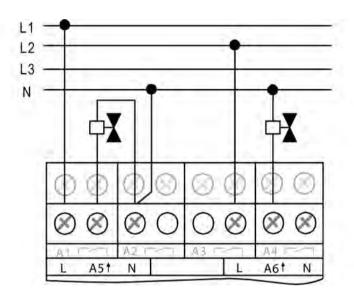
Figure 5: Electrical connection for electrothermal valve drives
