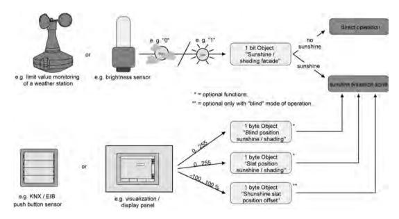
Figure 38: Schematic diagram illustrating the simple sun protection configuration
