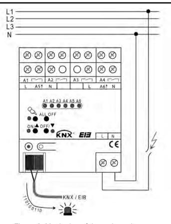
Figure 8: Monitoring of the mains voltage
