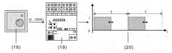
Figure 57: Command value principle with constant command value
