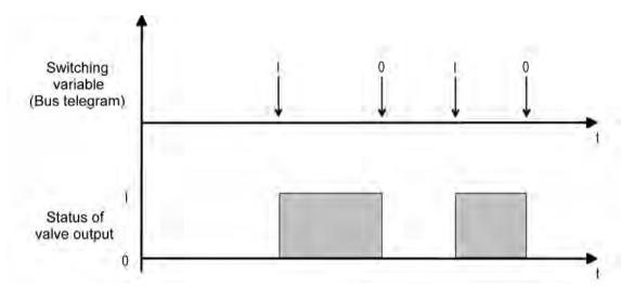
Figure 51: Conversion of a switching command value into an output signal with valve drives that are closed when deenergized (example)
