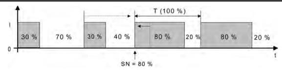
Figure 64: Command value change e.g. from 30 % to 80 % during the closing phase of the valve (closing phase too long)
