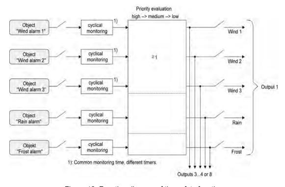
Figure 13: Function diagram of the safety function
