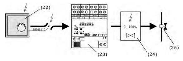
Figure 67: Principle of cyclical command value monitoring in the event of a fault (e.g. open circuit)
