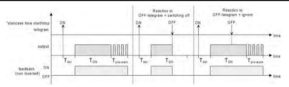
Figure 19: Switch-off behaviour of the staircase function
