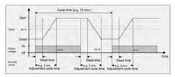
Figure 65: Idealised curve of the valve stroke: example for a command value of approx. 60 % for a valve closed when deenergized
