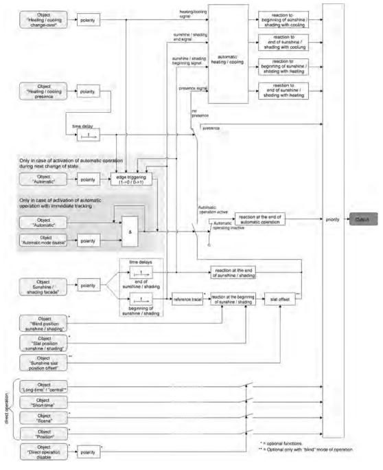
Figure 49: Function diagram of automatic heating/cooling
