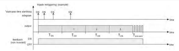
Figure 21: Time extension for staircase function
