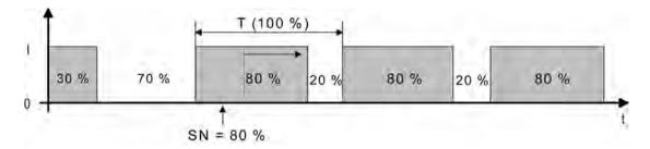
Figure 62: Command value change e.g. from 30 % to 80 % during the opening phase of the valve
