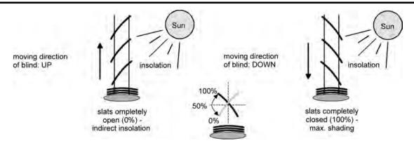
Figure 30: type 1 - slatted blinds with oblique slat position in both travel directions
