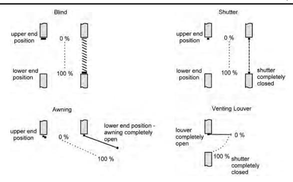
Figure 32: Positions defined as a function of the type of movement
