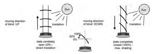
Figure 31: Type 2 - slatted blinds with oblique and horizontal slat position
