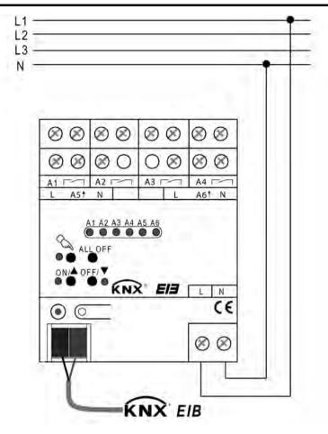
Figure 2: Electrical connection of mains voltage
