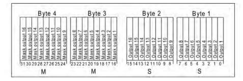
Figure 11: Structure of the centralized feedback object
