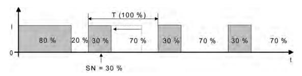
Figure 59: Command value change e.g. from 80 % to 30 % during the opening phase of the valve
