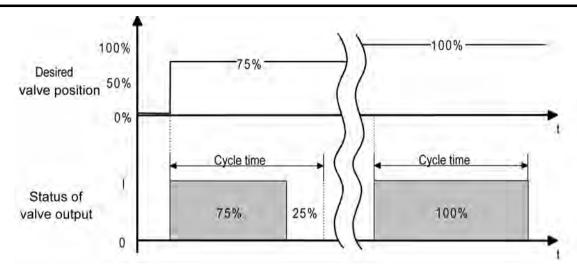
Figure 52: Conversion of a constant valve nominal position into an output signal with valve drives that are closed when deenergized (example)
