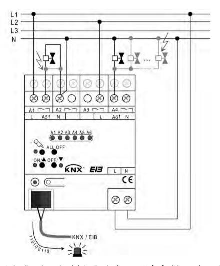
Figure 55: Short-circuit and overload detection in the event of a fault in a valve output or valve drive
