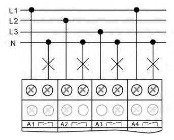
Figure 4: Electrical connection for loads in switching operation
