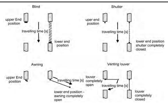
Figure 29: Travelling time as a function of the type of movement
