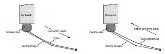
Figure 50: Fabric-stretching in an awning
