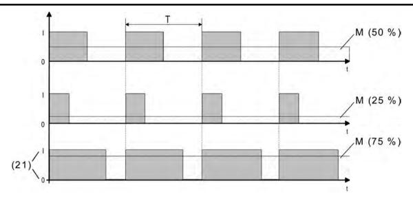
Figure 58: Pulse-width modulation of a valve output signal
