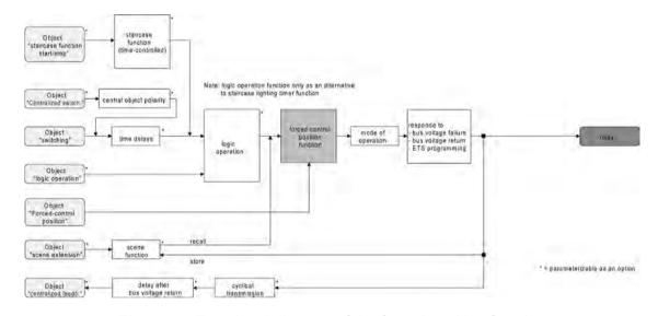
Figure 25: Functional diagram of the forced position function
