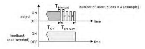
Figure 20: The pre-warning function of the staircase function (example)
