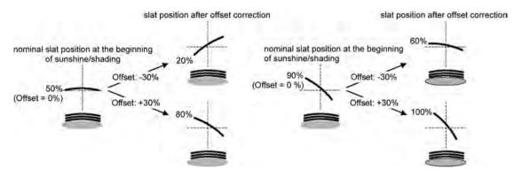
Figure 42: Functional principle of slat offset (typical of slat type 1; analogous reaction for slat type 2)
