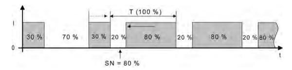
Figure 63: Command value change e.g. from 30 % to 80 % during the closing phase of the valve
