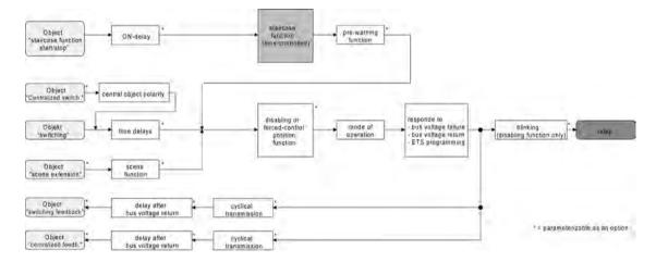
Figure 17: Functional diagram of the staircase function
