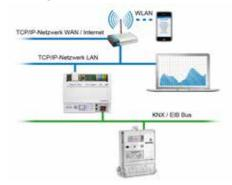
The integrated KNX data logger stores the data at 15 minute intervals over a period of The data can be read out one year. directly via the NK-FW network coupler using a standard Internet browser. Βv using FTP, you can also download the stored data from the KNX/EIB module for further processing, for example with MS Excel or Flash / Silverlight. The application program offers 15 data points for further processing in the KNX/EIB bus. The individual data can be transmitted cyclically to the KNX bus.
