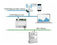
The integrated KNX data logger stores the data at 15 minute intervals over a period of one year. The data can be read out directly via the NK-FW network coupler using a standard Internet browser. By using FTP, you can also download the stored data from the KNX/EIB module for further processing, for example with MS Excel or Flash / Silverlight. The application program offers 21 data points for further processing in the KNX/EIB bus. The individual data can be transmitted cyclically to the KNX bus.
