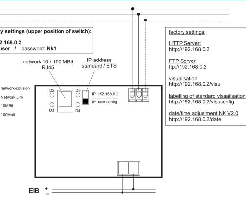
A slide switch in the upper part of the device allows the selection of the IP address:
