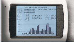
Every 15 minutes, the meter is read automatically and the readings are saved internally in a file for one year.
