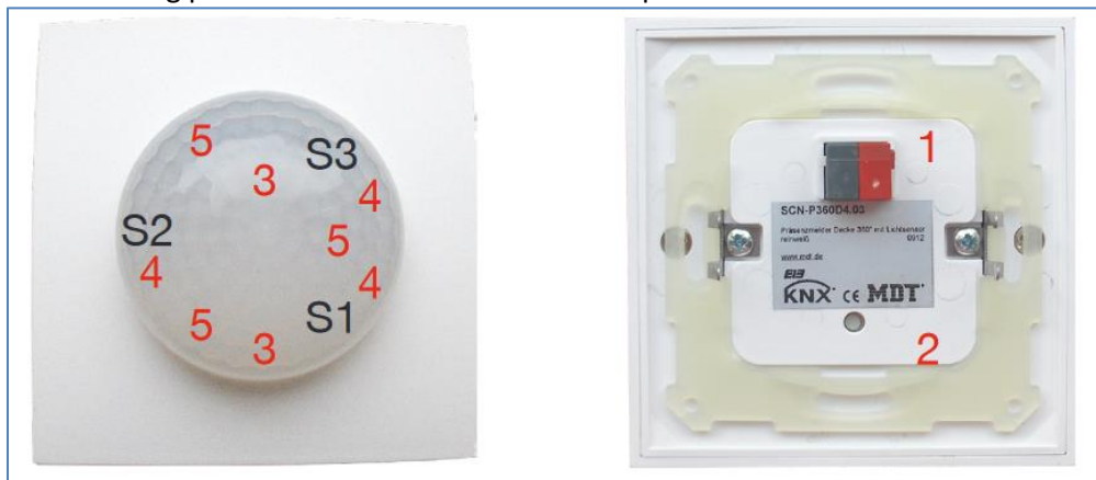
Figure 3: Structure and location of the sensors/LEDs – SCN-P/G360x3.03
