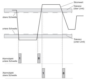
Using the alarm function, this means you can also visualise an undershoot of a defined current threshold. The reasons for this could be the failure of cooling installations, for example. You will then be alerted to this by an alarm telegram.
