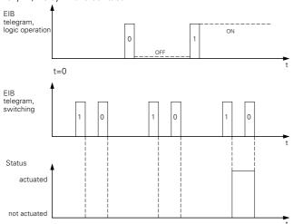
The logic object is preassigned the value "1" after a RE-SET. Switching can therefore be carried out as usual via the switch object. The closing lock-out is only active after the receipt of a "0" telegram via the logic object.
