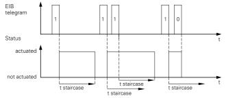
Non-retriggerable staircase lighting function with manual OFF function
