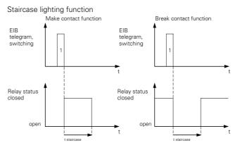
The period (t staircase) is calculated by multiplying a base value by a factor.
