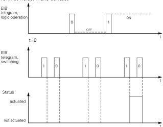
The parameter setting causes the "Logic object" to be set to the value "0". After a RESET, the actuator will not switch the output in the "make contact" mode nor with these settings, until a "1" telegram has been received at the "Logic object".
