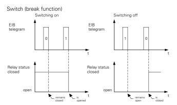
The fixed relay positions (open, closed) within the other functions are triggered directly. An inversion by means of the break contact function is no longer carried out for these fixed relay positions.
