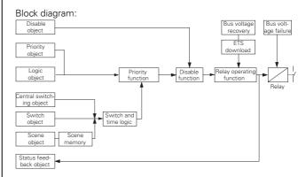
With regard to the switching behaviour of the actuator, each function has a certain priority. The weighting of the functions can be taken from the following table:
