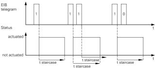
For the staircase lighting function, you can use the parameter "with / without manual OFF function" to set whether the timer is switched off prematurely after a
