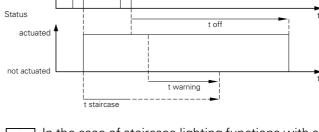
In the case of staircase lighting functions with a manual OFF function and active prewarning, the staircase lighting function with prewarning is immediately deactivated on receipt of an OFF telegram. The OFF delay elapses. No prewarning takes place.
