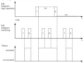
The relay can only be opened via the "Switch object" once a "0" telegram has been received via the "Logic object".
