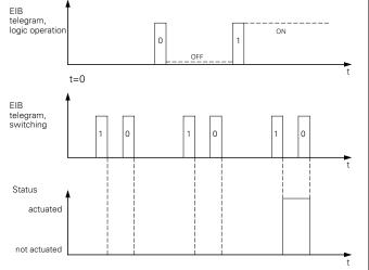
The parameter setting causes the "Logic object" to be set to the value "0". After a RESET, the actuator will not switch the output in the "make contact" mode nor with these settings, until a "1" telegram has been received at the "Logic object".
