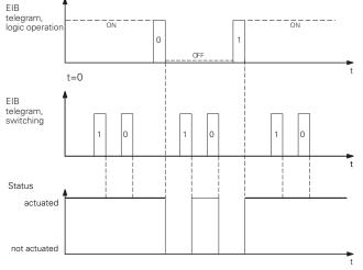
The logic object is preassigned the value "1" after a RESET. The actuator will immediately switch on the output in the "make contact" mode. The OR logic function is only reset by a "0" telegram at the logic object.
