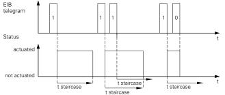
The staircase lighting function can indicate that the end of the staircase timer is imminent by causing the luminaire to flicker. It is possible to select between one and three warnings. It is possible to set the time (t warning) when the warnings should start before the staircase timer has elapsed. The length of the interruptions (t l) and the interval between two warnings (t int) can also be set.
