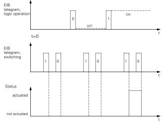
The logic object is preassigned the value "1" after a RE-SET. Switching can therefore be carried out as usual via the switch object. The closing lock-out is only active after the receipt of a "0" telegram via the logic object.
