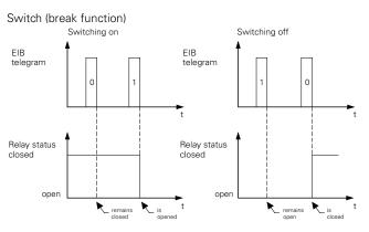
The fixed relay positions (open, closed) within the other functions are triggered directly. An inversion by means of the break contact function is no longer carried out for these fixed relay positions.
