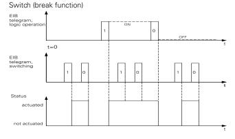
After bus voltage recovery, the relay is closed in the "break contact" mode and a status response telegram is generated with the value "1" if the status response function is activated. In this case, a different response is carried out e.g. by a higher priority function or due to the behaviour on bus voltage recovery at the output.
