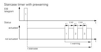
In the case of staircase lighting functions with a manual OFF function and active prewarning, the staircase lighting function with prewarning is immediately deactivated when an OFF telegram is received.
