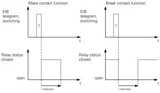
The period (t staircase) is calculated by multiplying a base value by a factor.
