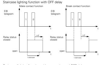
Staircase lighting function with prewarning and OFF delay
