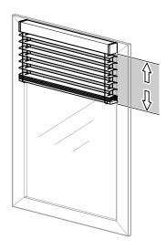
When the limit function is active, the drive only moves between the limit values. The limit applies for all movement commands from manual operation, automatic functions, scenes, presets and for movements from functions of lower priority.
