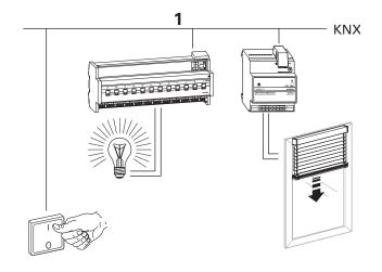
Blind actuator with manual actuation (and auxiliary power supply)
