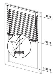
Step 2: Height running time = 24 s, upwards direction (Difference between current position 50 % and new position 30 % = 20 % of height running time) plus
