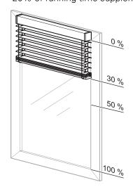
Step 3: Slat adjustment into the working position after upwards movement = **1.25 s** (Slat running time from 0 % to 50 %)
