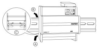
1 Place the blind actuator on the DIN rail from underneath (A) and push it upwards. Then press up (B) so that the claws on the rear side fix into the rail (C).
