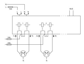
(6) Switch on the mains voltage for the motor. Now you can check that the blind actuator and connected motors work without having to load the application from the ETS (see section "Operation", "How manual operation works").
