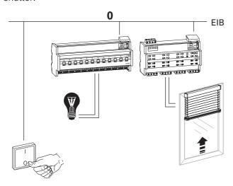
In this case, due to the fact that the roller shutter requires a certain running time to open, the light needs to be swiched off with a switch-off delay so that it doesn't suddenly become dark prematurely.
