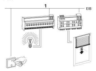
Blind actuator with manual actuation (without auxiliary power supply)
