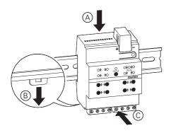
1) Place the blind actuator on the DIN rail.
