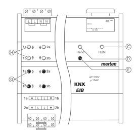
(1) Briefly press the manual operation key (E). The red manual operation LED (D) lights up. The actuator is in manual operation.
