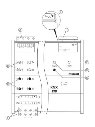
(A): Mains connection: The actuator has two connecting terminals each for the N and L cables (looping is possible).
