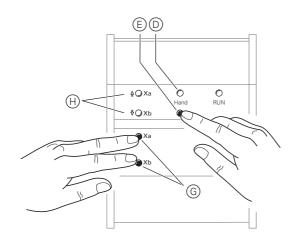
After 3 s, the manual operation LED  $\bigcirc$  flashes and the channel status LEDs H show the status of the channels.
