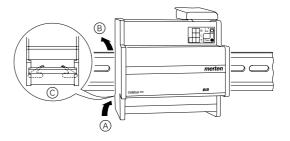
Place the actuator on the DIN rail from underneath
