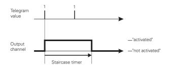
retriggerable: After a new telegram has been received with the object value "1", the staircase timer is restarted.
