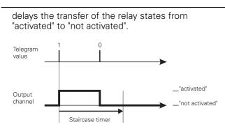
without manual OFF: A telegram with the object value "0" has no effects. The staircase timer set continues to run normally until the end. An OFF delay cannot be set.
