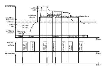
The additional lighting is switched on during the dimming-up phase since the dimmer alone cannot reach the setpoint value.
