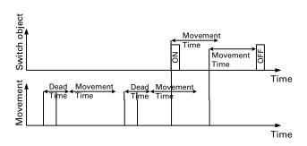
In master mode or normal mode the movement time corresponds to the staircase timer in the diagram above. In slave mode or monitoring mode the movement time corresponds to the cycle time. In practice a large number of applications can be implemented by means of the various blocks and sensors.
