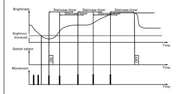
The movement detector changes to non-brightness-dependent mode once the start of movement action (sending an ON telegram) has been carried out. Here freshly detected movements can retrigger the staircase timer.
