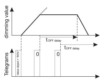
If the output receives a new telegram while an OFF delay is active, which creates an ON status, the OFF procedure will be halted and the new setpoint value set.
