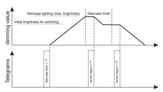
You can use this, for example, for temporary continuous light switching (cleaning lighting). An ON telegram from the switch object causes the light in the staircase lighting function to remain switched on continuously. Value, dimming, scene and central telegrams continue to be effective, however. For an application of this type, an initial brightness of 100% would be useful.
