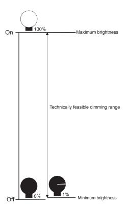
Use the software application to limit the technically possible dimming range to a minimum and a maximum dimming value. This limitation can be set individually for each output channel.
