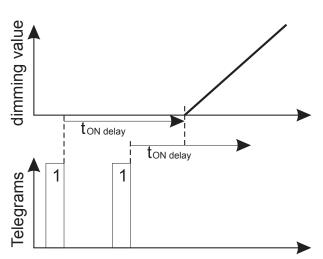
If the channel receives an OFF telegram while an ON delay is active, the ON delay will be interrupted.
