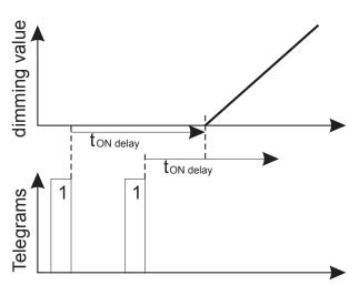
If the channel receives an OFF telegram while an ON delay is active, the ON delay will be interrupted.
