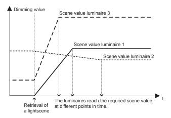
The "Same dimming time" function can be used to synchronise the different dimming times of the channels in such a way that all channels reach their setpoint value at the same time. Using the "Time factor modifiable via the bus" parameter (via the communication object "Factor same dimming time"), the dimming times can also be synchronised for several dimming actuators.
