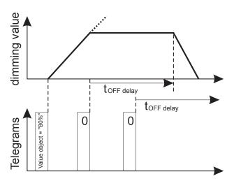
If the output receives a new telegram while an OFF delay is active, which creates an ON status, the OFF procedure will be halted and the new setpoint value
