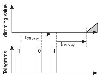
You can use a parameter to set whether the output channel remains switched off during the ON delay, or whether it is already set to the minimum dimming value.
