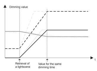
You can release the function globally for the device via a parameter, and set the corresponding dimming time after release:
