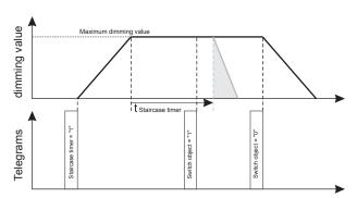
The brightness of the logic operation result and the dimming speed is defined by the last telegram (see the charts below).
