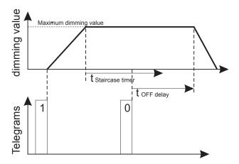
If you have selected the parameter value "without manual OFF", the staircase lighting function will not be interrupted when a telegram with the value "0" is received, but will continue to run normally until the staircase timer has expired.
