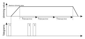
You can limit the potential running time using the "Max. number of time accumulations" parameter.
