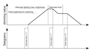
You can use this, for example, for temporary continuous light switching (cleaning lighting). An ON telegram from the switch object causes the light in the staircase lighting function to remain switched on continuously. Value, dimming, scene and central telegrams continue to be effective, however. For an application of this type, an initial brightness of 100% would be useful.
