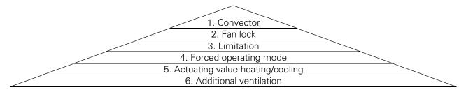
The heating system = convector / fan coil and cooling system = convector / fan coil parameters have the highest priority (1.). The fan is not actuated with the convector.
