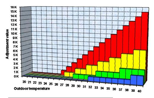
■1K per 7K outdoor temperature ■1K per 4K outdoor temperature ■1K per 2K outdoor temperature ■1K per 1K outdoor temperature
