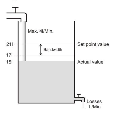
A filling volume of 15l gives rise to a control deviation of 211 - 151 = 61Because our actual value lies outside the bandwidth, the control will control the flow at 100% i.e. at 4l / minute
