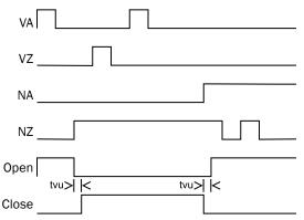
Louver blind mode: Local inputs are level-controlled for short button presses and edge-controlled for long button presses.
