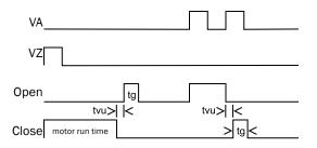
Operating mode Z with motor run time: Auxiliary inputs are edge-triggered and timer-controlled.
