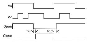
While auxiliary inputs are active, local inputs are ignored. NA has priority over NZ.
