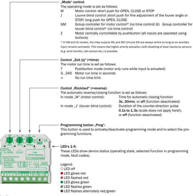
Local inputs for OPEN (VA) and CLOSE (VZ) push-buttons Auxiliary inputs for central/group control inputs OPEN (NA) and CLOSE (NZ)
