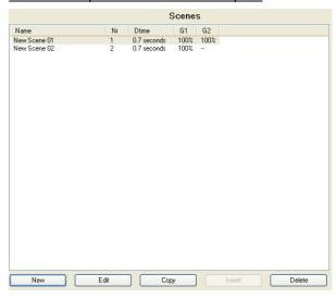
The "Scenes" parameter window enables an overview of how many scenes have already been configured and which groups are integrated in a scene in each case. When the cursor is placed in the first row under the column header "Name", a line appears explaining the abbreviations used in the header.
