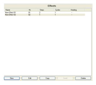
The "Effects" parameter window enables an overview of how many effects have already been configured and how many steps and run-throughs they consist of in each case.
