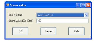
Via the "Scene value" window the group/ECG belonging to the scene can be changed, as well as assigned a dimming value (scene value) to which the group/ECG in this scene is to be set. If another group/ECG than the group/ECG displayed on opening of the window is selected via the "ECG/Group" parameter, this leads to the deleting (replacement) of the previous group/ECG in the respective scene.
