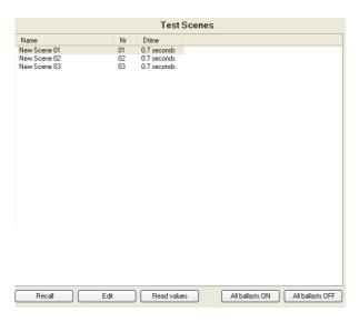
Double-clicking on a list entry or on the "Edit" button opens the parameter window for scene parameters.
