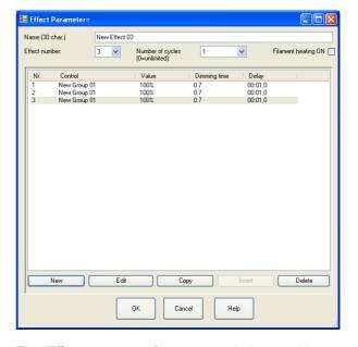
The "Effect, parameters" parameter window provides an overview of how many steps the effect consists of and what happens step by step: whether an individual ECG or a group are switched or dimmed or whether a scene is recalled and which interval should be observed following every step. If the cursor is placed in the header, a line appears explaining the abbreviations used in the header.
