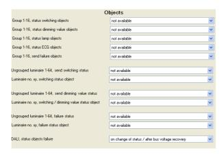
The basic functionality of the gateway can be expanded by additional communication objects via the "Objects" parameter window.
