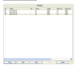
The "ECGs" parameter window enables an overview of how many DALI ECGs are attached to the Gateway and whether or, respectively, to which group an ECG has been assigned. When the cursor is placed in the first row under the column header "Nr.", a line appears explaining the abbreviations used in the header.
