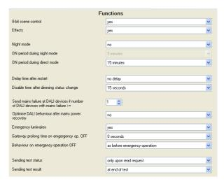
The basic functionality of the gateway can be expanded by additional functions via the "Functions" parameter window. This includes time-limited switching on of lighting during the night (cleaning light), 8-bit scene control integrated into the gateway, an additional control of light effects and the determination whether and how the various status objects are to be transmitted.
