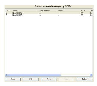
The parameter window "Self-contained emergency ECGs" enables an overview of how many DALI ECGs in emergency luminaires are attached to the Gateway and whether or, respectively, to which group an ECG has been assigned. When the cursor is placed in the first row under the column header "Nr.", a line appears explaining the abbreviations used in the header.
