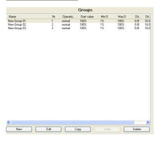
The "Groups" parameter window enables an overview of how many switching / dimming groups were assigned to the Gateway N 141/02. When the cursor is placed in the first row under the column header "Name", a line appears explaining the abbreviations used in the header.
