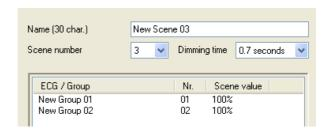
A new group or ECG can be added in the "Scene, parameters" window using the "New" button. Double-clicking on a list entry or on the "Edit" button the "Scene value" parameter window further down now opens. A marked group or ECG can be deleted in the "Scene, parameters" window with the "Delete" button.
