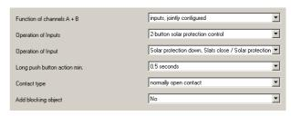
Using one push button pair, the solar protection can be lowered or raised to the respective final position with a long push button action, while a short push button action ends the movement or adjusts the slats by one step. An adjustment can be made to define which push button (or channel) is used to lower the solar protection and close the slats by one step where necessary, and which is used to raise the solar protection and open the slats by one step where necessary.
