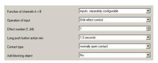
Using the 8-bit effect control it is possible to use a push button connected to the input to start and stop the effect with the configured number (1...64) on a KNX / DALI Gateway N141/02.
