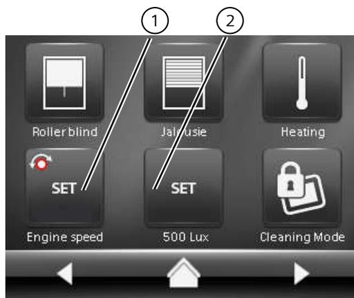
Figure. 22. Function page with "send value" buttons (example)
