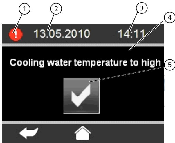
Figure. 27. Operating page with active alarm (example)
